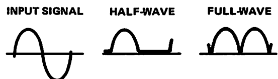
Figure 5-44. Rectifier Output-Voltage Waveforms
