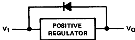
Figure 5-27. Reverse Bias Protection
